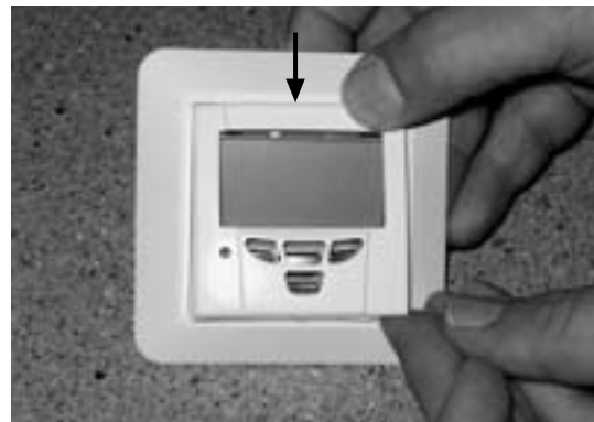
Fastening of the panel cover on the ILTO Premium controller: First set the upper edge of the cover in place, then press to fasten the cover in place
