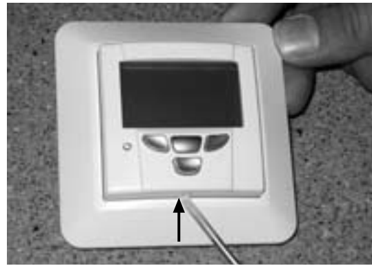
Loosening of the panel from the ILTO Premium controller
